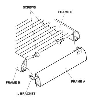
6. Install the remaining frame A to frame B the same way.
