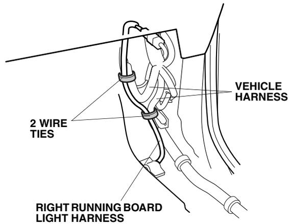
37. Check that all wire harnesses are routed properly and all connectors are plugged in.
