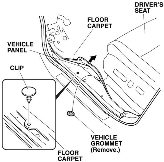
18. Remove the vehicle grommet of the vehicle panel.
