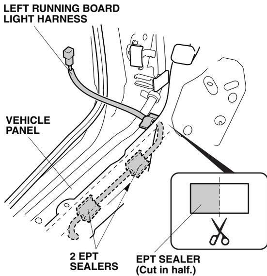
22. Using isopropyl alcohol on a shop towel, clean the areas where the EPT sealers will attach. Secure the left running board light harness to the vehicle panel with two EPT sealers.
