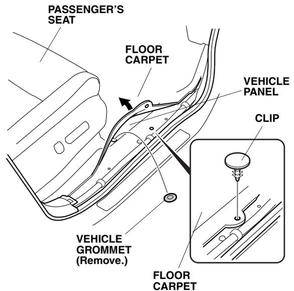
28. Remove the vehicle grommet from the vehicle panel.
