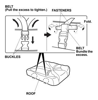
23. Bundle the excess belts on the buckles as shown and fold the fasteners inward to secure the belts on the buckles.
