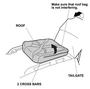
2. With the help from an assistant, carefully unfold the roof bag on the cross bars.
