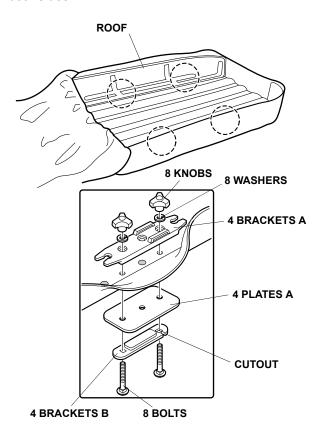
11. Loosely install bracket A, four plates A, and bracket B to the roof bag with two bolts, two washers, and two knobs for each location shown. Be sure the cutout on bracket B is facing the outboard side of the vehicle. 12. With the help from an assistant, carefully place the roof bag on the cross bar.
