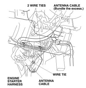
71. Bundle the excess of the antenna cable. Secure the antenna cable to the engine starter harness with two wire ties.
