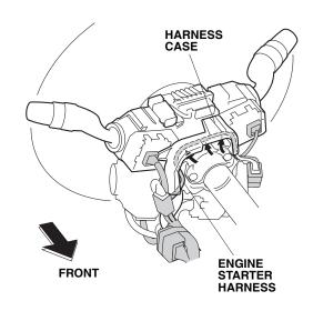
49. Secure the 12-pin and 8-pin connectors to the harness case with two wire ties.
