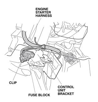
30. Install the engine starter harness clip on the vehicle bracket.
