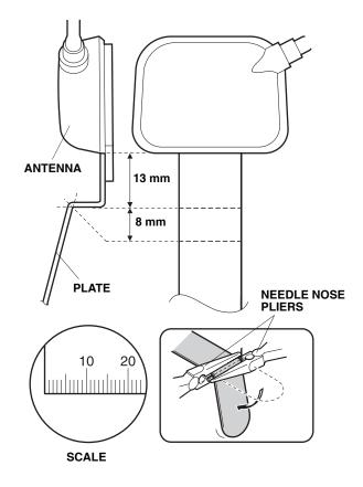
57. Starting near the antenna end of the cable, wrap three urethane tapes around the antenna cable at the measurements shown.
