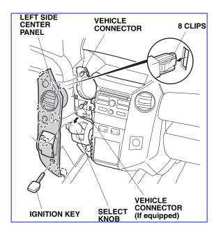
19. Remove the driver's dashboard lower cover (12 clips, one self-tapping screw and unplug the vehicle connectors). Remove the A/C sensor (two remaining tabs).
