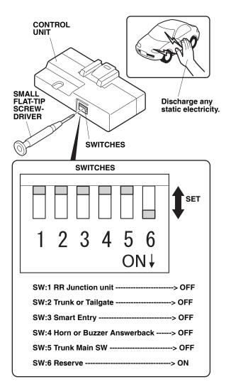
4. Check a location of the switches on the control unit. NOTE:
