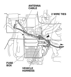
69. Route the antenna cable terminal to right side of the vehicle, and plug it to the control unit as shown.
