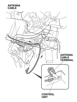
70. Secure the engine starter harness and antenna cable with one wire tie as shown.
