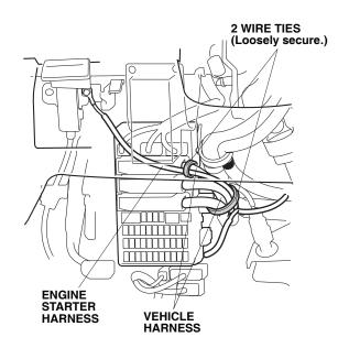
45. Route the engine starter harness 5-pin connector to the ignition switch.
