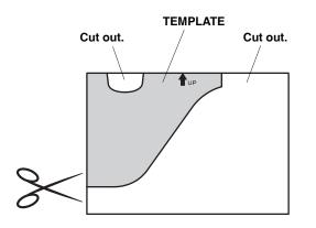
59. Secure the template to the windshield with masking tapes by aligning it with the edge of the black ceramic paint as shown.
