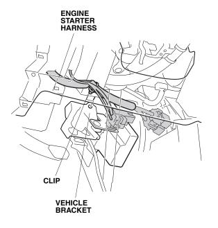
31. Route the engine starter harness relay block to the right side of the vehicle.
