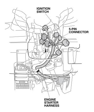
46. Unplug the vehicle 12-pin connector, and plug it into the engine starter harness 12-pin connectors. Plug the remaining engine starter harness 12-pin connector into the turn signal switch.
