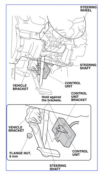
29. Install the engine starter harness fuse block clip on the control unit bracket.
