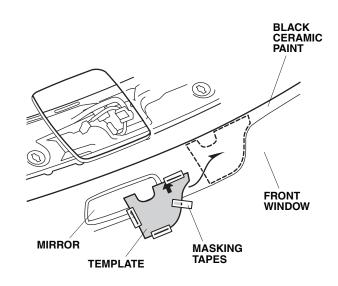
60. Using isopropyl alcohol on a shop towel, clean the area where the antenna will attach. Allow to dry before proceeding.
