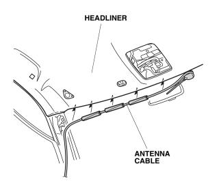
64. Clean the vehicle panel surface where the urethane tape will attach with isopropyl alcohol. Secure the antenna cable to the vehicle panel with the smaller part urethane tape that you cut into two in step 40. Be careful not to crease the headliner.
