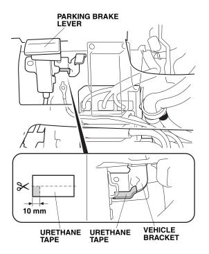
41. Clean the vehicle bracket surface where the urethane tape will attach with isopropyl alcohol. Attach the urethane tape that you cut in step 40 to the vehicle bracket as shown.
