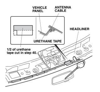
65. Clean the vehicle panel surface where the urethane tape will attach with isopropyl alcohol. Secure the antenna cable to the vehicle panel with the remaining part of the urethane tape you cut in step 40. Be careful no to crease the headliner.
