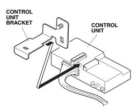
28. Secure the control unit to the vehicle bracket with a 6 mm flange nut.
