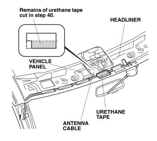
66. Route the antenna cable along the left A-pillar and secure the antenna cable to the vehicle harness with four wire ties as shown.
