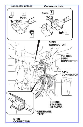
51. Plug the engine starter harness 5-pin connector into the vehicle 5-pin connector.
