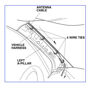
67. Secure the antenna cable to the vehicle harness with one wire tie.
