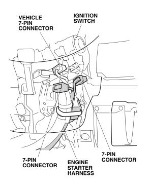
55. Secure the engine starter harness to the vehicle harness with one wire tie as shown.
