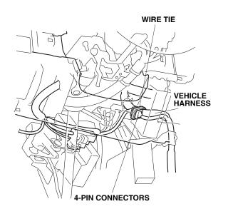
35. Align the green-taped part of the engine starter harness with the vehicle clip. Secure the engine starter harness to the vehicle harness with one wire tie.
