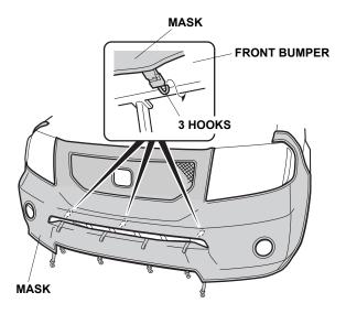
9. Route the four upper straps of the mask through the inside of the front bumper, and attach the four hooks to the loop on the four upper straps of the mask as shown.
