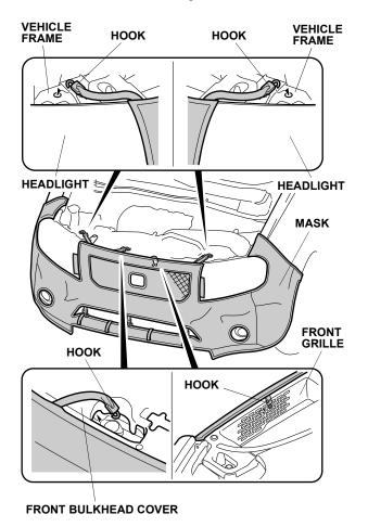
7. Insert the tab on each side between the front grille and the headlight.
