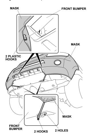
11. Attach the two hooks to the bottom holes of the front bumper as shown.
