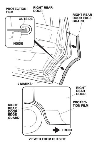
15. Tap the right rear door edge guard into position with a series of light taps using a rubber mallet. Make sure the position is correct. Once in place, do not remove, reposition, or reinstall the right rear door edge guard or it will not hold securely.
