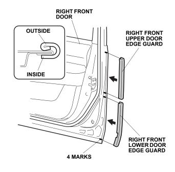
8. Tap the right front door edge guards into position with a series of light taps using a rubber mallet. Make sure their positions are correct. Once in place, do not remove, reposition, or reinstall the right front door edge guards or they will not hold securely.
