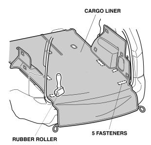
8. Align the cargo liner to the right rear side panel, fold the cargo liner over and using the two alcohol swabs, throughly clean the area where the loop fasteners will attach.
