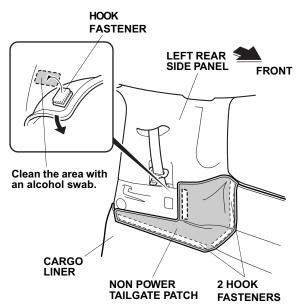
27. Align the non power tailgate patch to the left rear side panel, fold the non power tailgate patch over and using the alcohol swab, throughly clean the area where the hook fasteners will attach.
