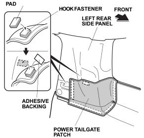
25. Remove the adhesive backing from two loop fasteners, fold the power tailgate patch over, and attach the two loop fasteners to the left rear side panel. Press the two loop fasteners firmly against the side panel with the rubber roller. Go to step 30.
