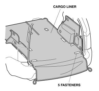
6. Attach five fasteners on the cargo liner to the cargo floor as shown.
