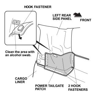
23. Align the power tailgate patch to the left rear side panel, fold the power tailgate patch over and using the alcohol swab, throughly clean the area where the fasteners will attach.
