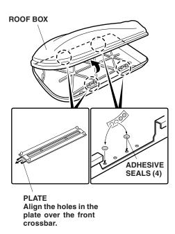
Attach an adhesive seal over the unused rear mounting holes along the bottom of the roof box.
