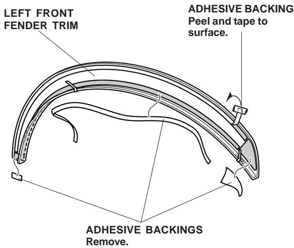
3. Using an alcohol swab, thoroughly clean the area where the left front fender trim will attach. Align the tip of the left front fender trim with the edge of the masking tape as shown.
