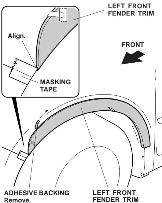
4. Attach the left front fender trim to the left front fender. While applying light pressure against the left front fender trim, carefully remove the taped adhesive backing.
