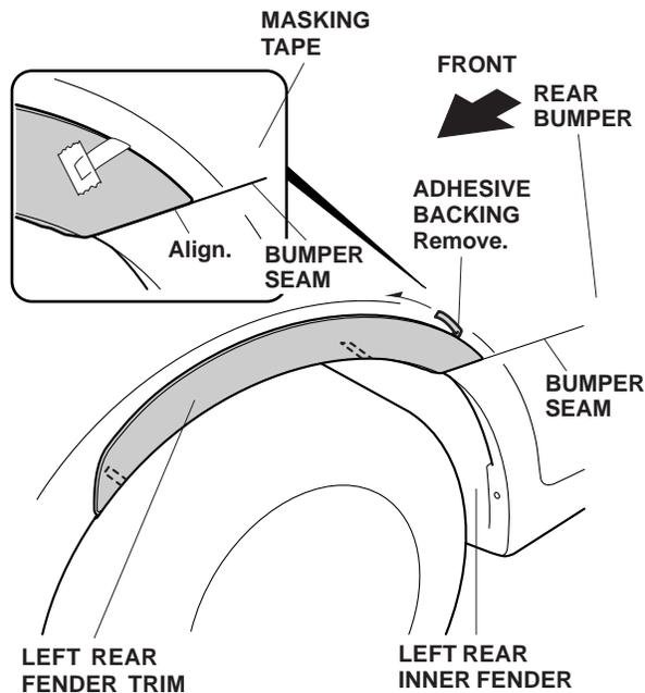
10. Peel back the adhesive backing from the upper part of the left rear bumper trim and tape it to the surface. Remove the remaining adhesive backings from the left rear bumper trim.
