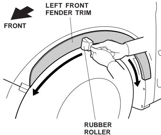
6. Hold the left front fender trim upward, and push the fender liner out of the way. Bend the two mounting tabs around the left front fender. Use needle-nose pliers wrapped in a shop towel to bend the mounting tabs around the fender flange.
