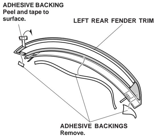
9. Using an alcohol swab, thoroughly clean the area where the left rear fender trim will attach. Align the edge of the left rear fender trim with the bumper seam as shown. While applying light pressure against the rear fender trim, carefully remove the taped adhesive backing.
