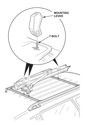
Position the bike attachment on the front and rear crossbars. Turn and adjust the mounting lever to lock the bike attachment to the roof rack. Check for firm pressure while you push down on the mounting lever to lock it into place.
