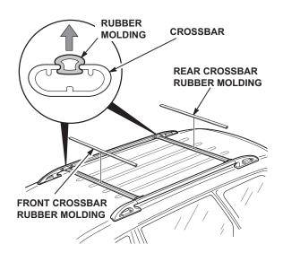
3. Remove the roof rack assembly from the roof (eight Phillips screws). Leave the adapter blocks in their original positions.
