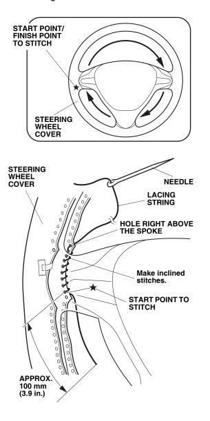
6. Stitch twice at the hole right above the spoke, and pull the lacing string to close the seam securely. Pull the lacing string securely to bring both ends of the steering wheel cover together very closely.
