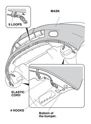
15. Attach the four hooks to the lower grille opening. Attach the eight plastic hooks to the bottom edge of the lower grille.
