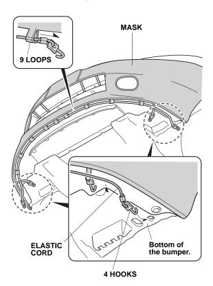
Attach the two hooks to the lower grille opening.
