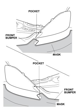
8. Insert four tabs into the opening between the front grille and the front bumper.
