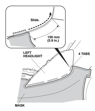
11. Repeat step 10 to install the mask on the right side of the vehicle.
