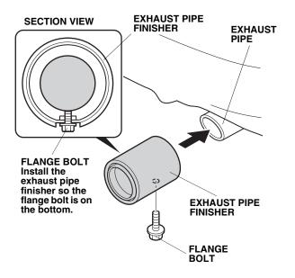
2. Slide the exhaust pipe trim onto the exhaust pipe until it bottoms against the exhaust pipe.
