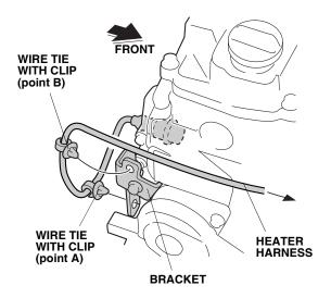
14. Route the heater harness as shown. Using two black wire ties, secure the heater harness to the vehicle harness.
