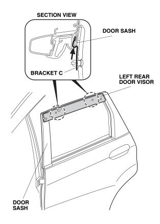
29. Insert bracket D between the rear pillar trim and the door sash, and insert the bracket E between the rear door center trim and the door sash. Install the left rear door visor on the door sash using the two clips. Verify the shape and the identification mark stamped on each bracket.
