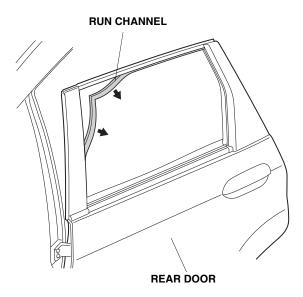
13. Remove the rear door run channel in the area shown.
