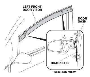
7. Push the left front door visor forward and up, and check that it aligns with the contour of the door sash. There should be no clearance between the brackets and the door sash.
