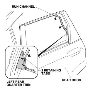
19. Carefully release the rear door run channel in the area shown. The run channel can tear easily at the corner area.
