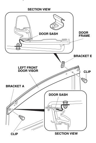
9. Adjust bracket A up or down until the hole in the bracket lines up with the hole in the door visor, and install a clip.
