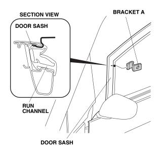
6. Temporarily install the left front door visor on the door sash using the two brackets C you installed on the left front door visor.
