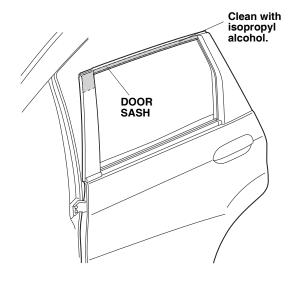
27. Temporarily install the left rear door visor on the door sash using the two brackets C you installed on the left rear door visor.
