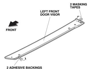
(Peel back 11/2 to 2 inches and tape to the front surface of the door visor.)
