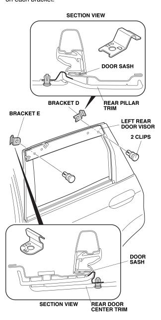
30. While holding the door visor up firmly and aligned in the center, remove the adhesive backings. Use your finger to push up on each bracket so there is no gap between the brackets and the door sash.
