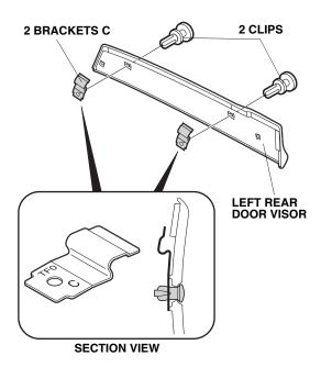
25. Peel back approximately 1½-2 inches of adhesive backing from each adhesive tape, and tape the ends to the front surface of the left rear visor.
