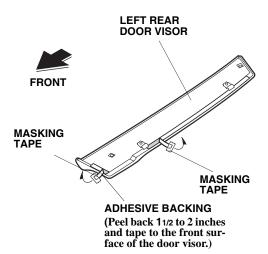
26. Using isopropyl alcohol on a shop towel, clean the door sash where the left rear door visor will attach.
