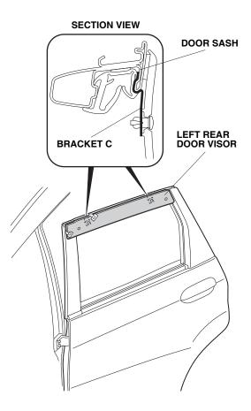
28. Push the left rear door visor upward, and check that it aligns with the contour of the door. There should be no clearance between the bracket and the door sash.
