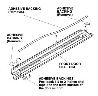
4. Clean the surface where the front door sill trim will be installed using an alcohol swab.
