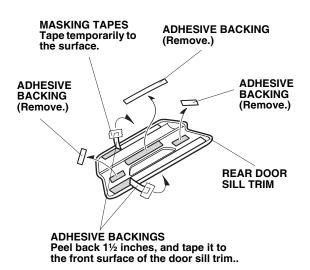
11. Clean the surface where the rear door sill trim will be installed using an alcohol swab.
