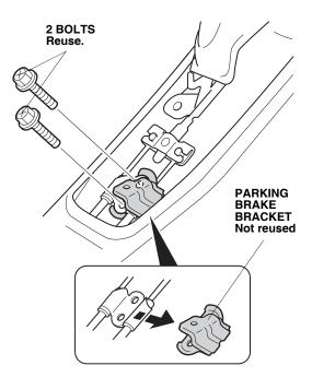
Install the floor bracket under the parking brake cables and reinstall the two bolts. Torque the bolts to 22 N·m (16 lb·ft). Be careful not to strip the threads.
