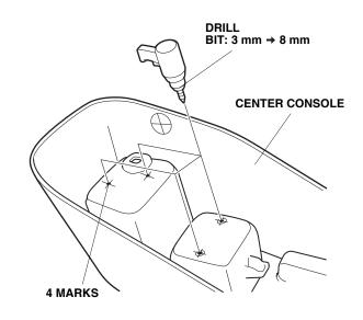
12. While wearing eye protection, drill the two pierced marks on the sides of the center console to 20 mm. First drill with a 3 mm drill bit, and finish with a 20 mm hole saw. Remove any burrs from the edge of the holes with a file.
