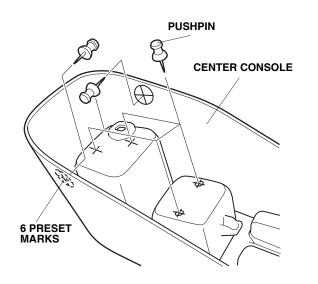
11. While wearing eye protection, drill the four pierced marks on the inside of the center console to 8 mm. First drill with a 3 mm drill bit, and finish with an 8 mm drill bit. Remove any burrs from the edge of the holes with a file.
