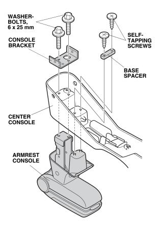
14. Install the base spacer to the armrest console using two self-tapping screws.
