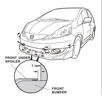
16. Using a rubber roller, apply firm pressure while rolling to set the adhesive.
