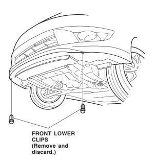
7. With the help of an assistant, temporarily install the front under spoiler to the front bumper using four self-tapping screws into the front fenderwell (two on each side) and two new clips under the spoiler.
