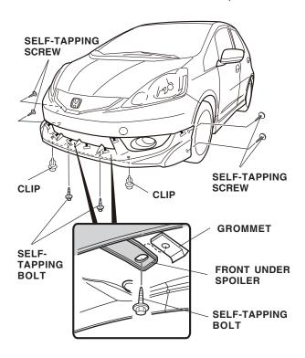
15. Make sure the front under spoiler is positioned properly on the front bumper with a 1 mm gap shown. Then, starting in the middle, slowly remove the lower adhesive backing while pushing inward. Remove the upper adhesive backing while gently lifting the under spoiler.
