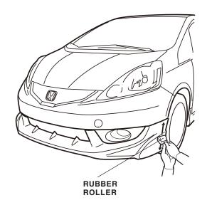
17. Tighten the self-tapping screws and bolts loosely installed in step 14. If there is a gap between the front bumper and the front under spoiler, use a 1 mm shim to close the gap. In some cases you may need to add two 1 mm shims to close the gap. Do not add more than two shims under each screw.
