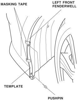
Using a pushpin, pierce the front fenderwell at the 2. two marks indicated on the template.
