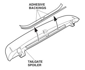
14. Using isopropyl alcohol, clean the tailgate area where the adhesive tape will attach.
