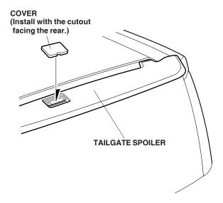
20. Press down and hold the tailgate spoiler at the adhesive tapes to the tailgate for 30 seconds.
