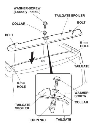
15. Position the tailgate spoiler on the tailgate and insert the two bolts into the 8 mm holes in the tailgate. Loosely install the washer-screw and the collar through the center hole in the tailgate spoiler and into the turn nut. Be careful not to drop the bolts on the vehicle.
