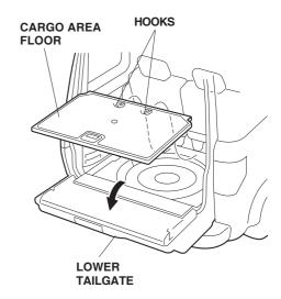
Raise the tailgate lower trim and remove the three self-tapping screws that fasten the tailgate lower trim. Remove the lower trim (two clips).
