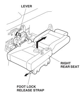
Push the lever in the direction shown, then remove the right rear seat by lifting the rear of the seat and sliding the seat towards the rear of the vehicle. 9. Remove the tie-down hook from the right rear side trim panel (one screw).
