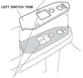
Check that the hole in the switch trim is aligned with the switch hole.
