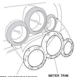
OUTER ADHESIVE BACKING Peel back 2 to 3 cm (1/2 to 1 in.) from the end, and tape it to the front of the trim.
