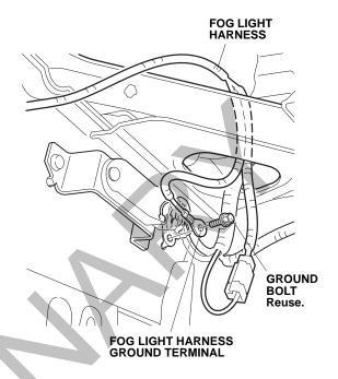
19. Secure the fog light harness 1-pin connector to the vehicle harness with one wire tie. Do not secure the 1-pin connector to the SRS harness with the wire tie.
