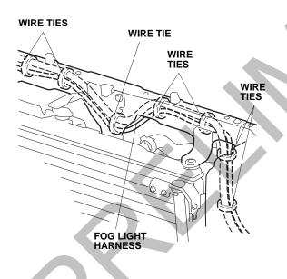
27. Secure the fog light harness to the vehicle harness with one wire tie at the green tape.
