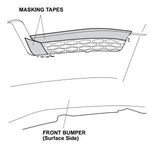
7. On the inside of the bumper, drill the two upper pierced marks to 25 mm. While wearing eye protection, first drill with a 3 mm drill bit and finish with a 25 mm hole saw.
