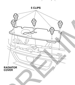
4. With the help of an assistant, remove the front bumper (five clips, four stepped bolts, and four self-tapping screws). Place the front bumper on the blanket to prevent damage.
