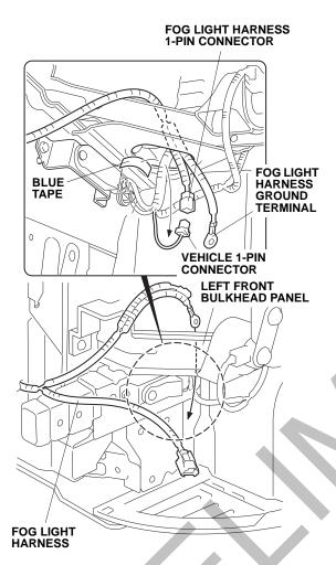
17. Locate the 1-pin connector blue-taped to the vehicle harness and remove the blue tape to free the 1-pin connector. Plug the 1-pin connector you just freed to the fog light harness 1-pin connector.
