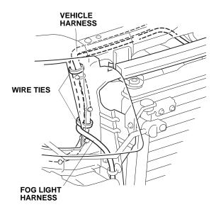
26. Secure the fog light harness to the vehicle harness with the seven wire ties in the areas shown.
