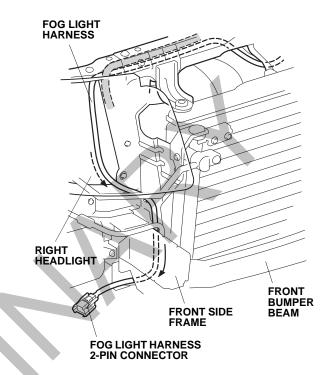
23. Push the two clips on the fog light harness into the holes in the bulkhead side stay.
