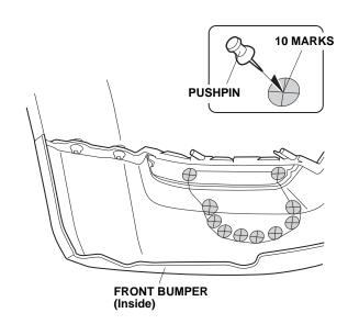
6. On the surface side of the bumper, attach masking tape to the bumper in the areas shown.
