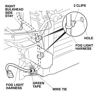
24. Secure the fog light harness to the vehicle frame with one wire tie at the green tape.
