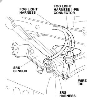
20. Behind the front side frame, route the fog light harness 2-pin connector (short end) down, and out through the clearance between the side frame and front bumper beam.
