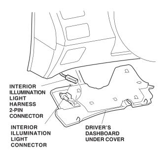
56. Plug the interior illumination light harness 2-pin connector to the interior illumination light connector on the lid of the dashboard center lower cover, and reinstall the lid.
