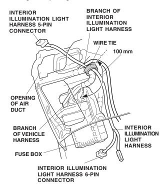
12. Measure the vehicle harness from the point of branch as shown. Secure the interior illumination light harness (6-pin connector side) to the vehicle harness with one wire tie.
