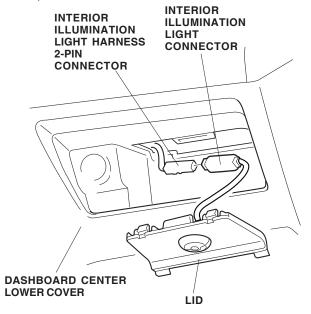
57. Plug the interior illumination light harness 2-pin connector to the interior illumination light connector on the passenger's dashboard under cover, and reinstall the under cover.
