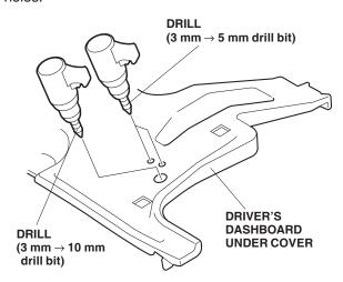
30. Cut the rib of the driver's dashboard under cover as shown. Using a file, remove any burrs from the edge.
