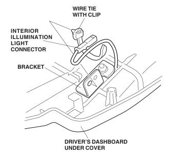
33. Reinstall the insulator to the driver's dashboard under cover, and pass the interior illumination light connector through the slit.
