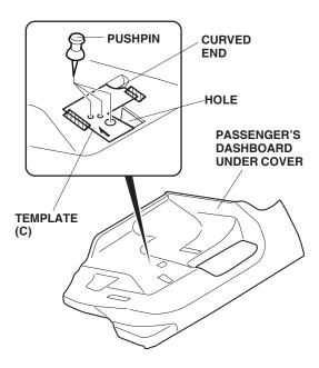
40. Using a pushpin, pierce the template at the three marked points. Remove the template.
