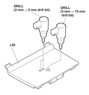
37. Route the interior illumination light (with blue tape) connector through the 10 mm hole. Install the courtesy light on the lid with the screw and flange nut.
