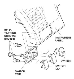
50. Install the switch and two switch lids to the switch trim. Go to step 53.
