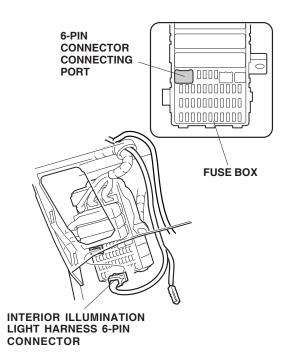
NOTE: If another accessory is already plugged into the 6-pin connector, remove the dummy connector from the other accessory harness, and plug the interior illumination light harness into that connector.
