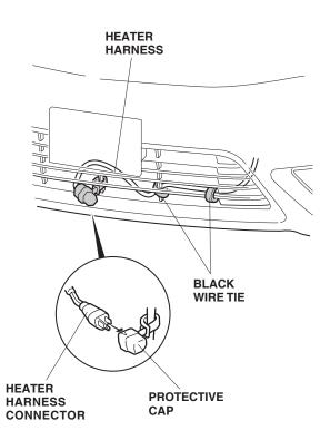
13. Attach the protective cap to the grille, and plug the connector of the heater harness into the protective cap.
