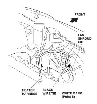
10. Secure a wire tie with clip, attached at point C, to the vehicle frame and route the heater harness to the front bumper opening.
