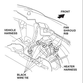
12. Route the heater harness inside the bumper and secure it with four black wire ties.
