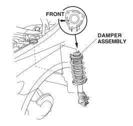
9. Loosely install the new flange nuts.
