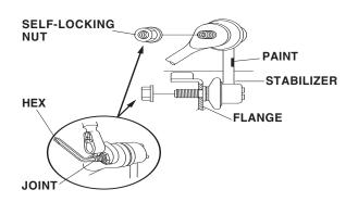
22. Remove the flange bolt that connects the knuckle and the upper arm.
