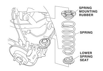
29. Align the bottom of the spring and the lower spring seat with the trailing arm as shown.
