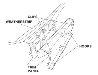
• Remove the clips, then remove the left trunk side trim panel from the trunk. Release the rear seat-back release cable out through the slit in the trim panel.
