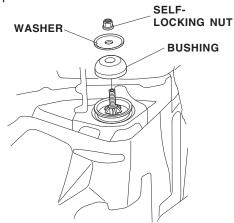
Torque the damper shaft self-locking nut to 29 N⋅m (21 lb-ft) while holding the damper shaft with a hex wrench.
