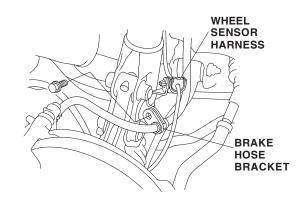
3. Remove the damper pinch bolts and self-locking nuts from the damper. Do not allow the knuckle to rotate too far outward. This may allow the inner CV joint bearing to unseat.
