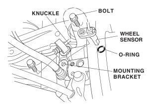
20. Remove the brake hose mounting bracket.
