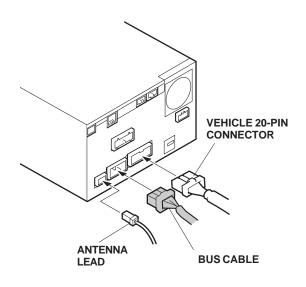
41. Connect the four vehicle connectors to the center panel, and reinstall the center panel.
