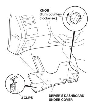
14. Release the eight clips, and remove the driver's dashboard lower cover by pulling it toward you. Take care not to damage the clips.
