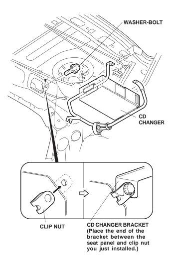
37. Slide the two clip nuts onto the CD changer brackets and rear shelf through the holes in the parcel shelf, and align their holes as shown. Install the two washer-bolts, and tighten them securely.
