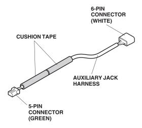
Locate the vehicle 6-pin connector blue taped to the vehicle connector. Remove the blue tape to free the connector. Plug the auxiliary jack harness 6-pin connector into the vehicle harness 6-pin connector.
