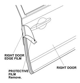
11. Starting from the middle and working outward, turn back the right door edge film half to the cabin side of the right door as shown. Move your fingers in one direction only.
