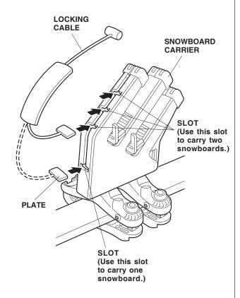
15. After loading each snowboard on to the carrier, adjust it with the help of the board supports so that the top edges are level and the boards are as far down in the carrier as possible. To secure the snowboard, use the key to open the covers, then insert the locking cable stoppers into the holes of the carrier covers.
