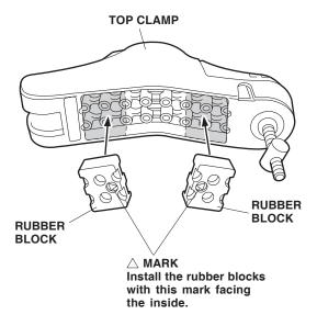
$\triangle$  MARK Install the rubber blocks with this mark facing the inside.
