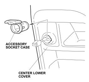
7. Slide the ring into the hole in the center lower cover in the direction shown.
