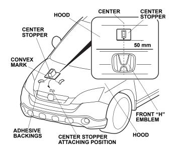
7. Remove the adhesive backing from the center stopper, and attach it to the hood at the marked location with the convex mark facing down.
