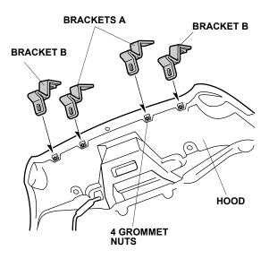
10. Close the hood. Attach a piece of masking tape to the hood under each bracket.
