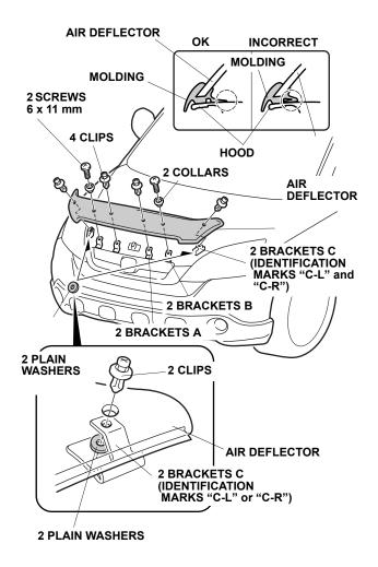
15. Align the holes in the air deflector over the two brackets B, and install the two screws and two collars. Tighten the screws securely. Check that the edge of the air deflector molding is seated properly.
