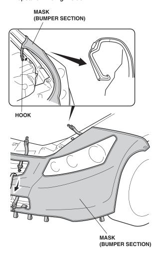
8. Pull the mask (bumper section) back toward the wheelwell, smooth out any wrinkles, and then snap the mask (bumper section) onto the snap-screw.
