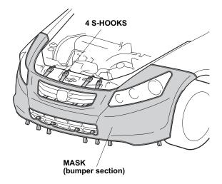
15. Attach the four plastic hooks to the bottom inside edge of the front bumper.
