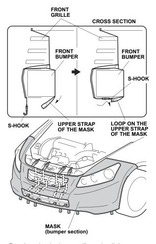
13. Reach under the lower grille and pull the straps out. Attach the four straps to the four hooks on the bottom of the mask.
