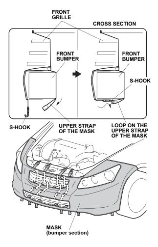
12. Route the four straps through the openings in the upper grille area, and down behind the bumper.
