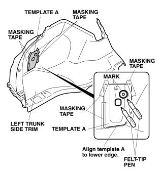
7. Using a felt-tip pen, mark the left trunk side trim as indicated on the template. Remove the template.
