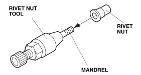
• Insert the rivet nut into the upper hole in the left trunk side panel, and install the hex wrench.
