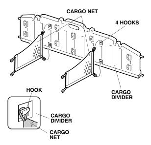
22. Slide the four pins from the cargo divider into the upright supports. Attach the cargo nets to the anchors on the rear trim panel. The cargo divider can be installed in two different positions:
