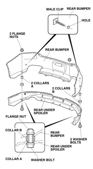
20. Secure the rear under spoiler to the rear bumper using four clips and two clip retainers as shown.
