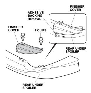
15. Press the finisher cover firmly while removing the adhesive backing that you temporarily attached to the surface side of the finisher cover.
