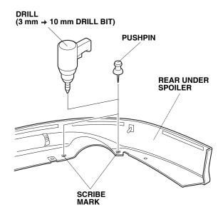
12. While wearing eye protection, drill a 3 mm hole through the mark from the rear under spoiler as shown. Finish with a 10 mm bit. Remove all burrs.
