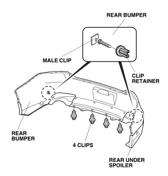
21. Secure the rear under spoiler to the rear bumper using four 5 x 14 mm self-tapping screws and four plain washers as shown.
