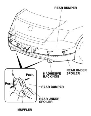
25. With a rubber roller, apply firm pressure while rolling to set the adhesive.
