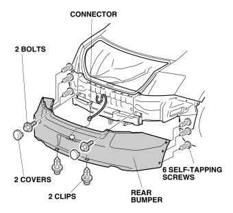
For L4 with a finisher cover, go to step 2. For V6, go to step 3.
