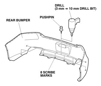
8. While wearing eye protection, first drill a 3 mm hole through the eight scribe marks from the inside of the rear bumper as shown. Finish with a 10 mm bit. Remove all burrs.
