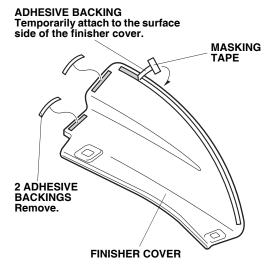
14. Position the finisher cover on the rear under spoiler, and install the two clips.
