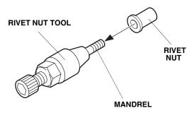
• Insert the rivet nut into the hole in the left trunk side panel, and install the hex wrench.
