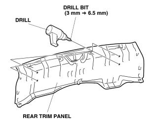
25. Install the four small anchors to the trunk rear trim panel using one 6 x 16 mm hex bolt, one 6 mm spring washer, and one 6 mm plain washer for each anchor. Torque the 6 x 16 mm hex bolts to 5 N·m (3.7 lb-ft). Position each anchor horizontally as shown.
