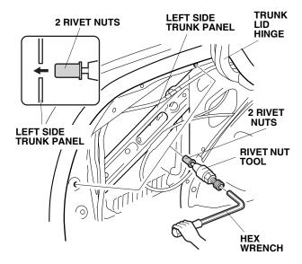
While holding the rivet nut tool with the hex wrench, use a 19 mm wrench to rotate the tool in a clockwise direction until the rivet nut is fully collapsed.
