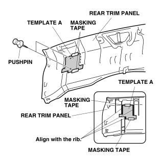
21. Using a pushpin, mark the back of the trunk rear trim panel according to template A. Remove the template.
