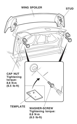
6. Remove each of the backings, then hold the wing spoiler firmly against the trunk lid with the palm of your hand, especially at the edges.
