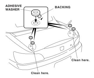
3. On the back of the wing spoiler, peel back 1 to 1½ inches of the backings from the adhesive tapes, and tape them to the front of the trunk spoiler with masking tape.
