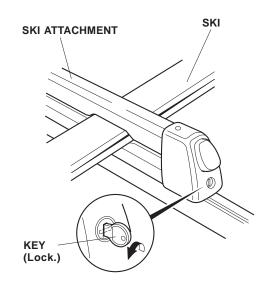
With the ski attached, rock the attachment in all directions to make sure it is installed securely. Adjust as necessary.
