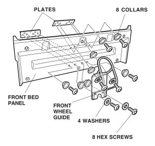
6. Reinstall the front bed panel and the upper tiedown hooks.
