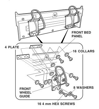
9. Reinstall the front bed panel and the upper tiedown hooks.
