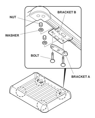
11. Position the roof basket on the roof rack, with the flap from frame A facing forward. Attach the basket to the cross bars by sliding bracket A around the crossbar and tightening the nuts. Tighten the nuts evenly.
