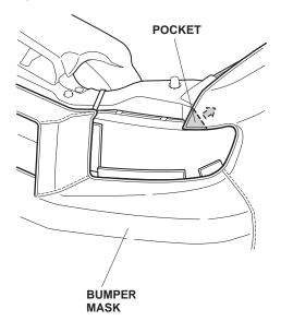
9. Attach the plastic clip to the top inside edge of the fender. Fit the mask across the bumper.
