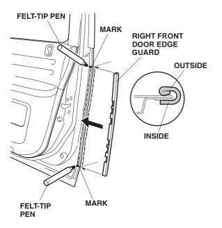
door edge, and tap it into position with a series of light taps using a rubber mallet.
