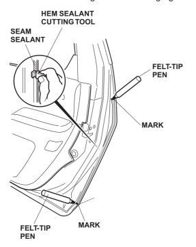
9. Position the hem sealant cutting tool against the door edge, and trim the seam sealant from mark to mark.
