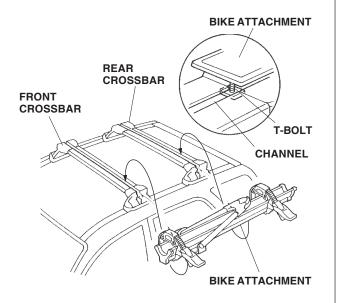
6. Turn and adjust the mounting levers to lock the bike attachment to the roof rack. Check for firm pressure while you push down on the mounting lever to lock it into place.
