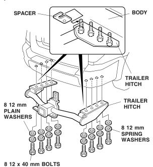
33. Insert one spacer on each side between the trailer hitch and the body at the rear bolts. Do not tighten the trailer hitch bolts at this time.
