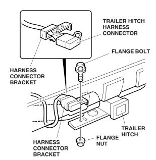
37. Secure the trailer hitch harness to the trailer hitch with two wire ties in the areas shown.
