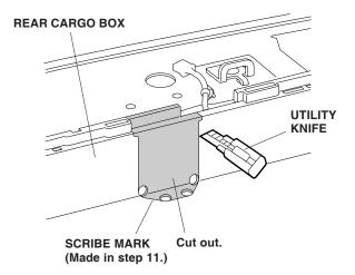
15. Using a utility knife, cut one cushion tape into four pieces. Attach small pieces to the converter bracket in the four locations shown. Be careful not to cover the holes in the bracket. Use isopropyl alcohol to clean the area where the cushion tapes will attach.
