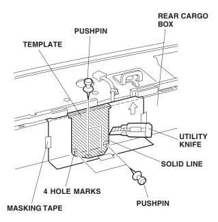
12. Using a pushpin, mark the rear cargo box at each of the four marks on the template. Using a utility knife, scribe the rear cargo box along the solid line on the template.
