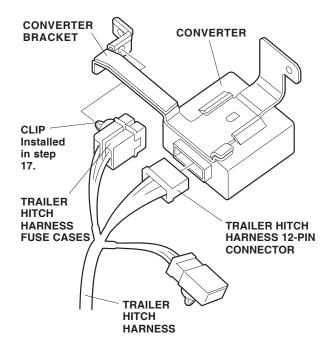
21. Push the clip installed from the trailer hitch harness fuse case into the hole in the converter bracket.
