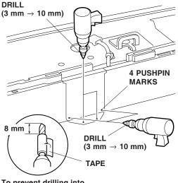
To prevent drilling into the frame, apply tape to the end of the drill bit
