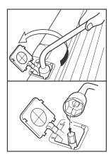
30. Under the rear bumper, locate the excess tabs. Using diagonal cutters, remove the tab and a small piece from the corner on the left side of the rear bumper in the area shown. Remove the tab and the corner piece from the right side of the rear bumper the same way.
