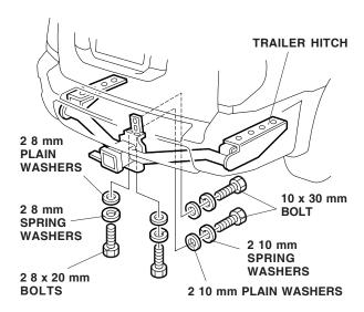
35. Torque the trailer hitch mounting bolts in this order:
