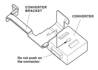
20. Plug the trailer hitch harness 12-pin connector into the converter.
