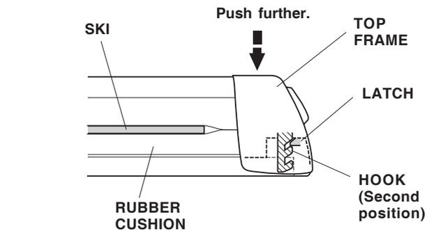
4. Lock the top frame by turning the key counterclockwise. Remove the key.
