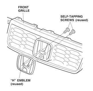
6. Insert the ribs of the front grille into the grooves of the front bumper, then attach the ends of the retaining tabs to the edge of the front bumper. Install the five clips.
