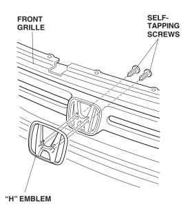
5. Attach the "H" emblem to the new front grille with the two self-tapping screws you removed.
