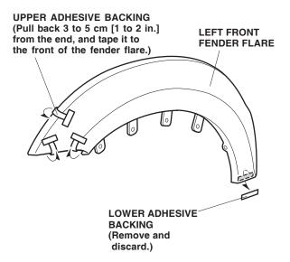
10. On the inside of the left front fender flare, pull back 3 to 5 cm (1 to 2 in.) from the upper and front adhesive backings. Fold the ends back, and tape them to the front of the fender flare. Remove and discard the two lower adhesive backings. 11. Align the ends of the front fender flare with the front edge of the front fender, and bend the mounting tabs around the fender flange.
