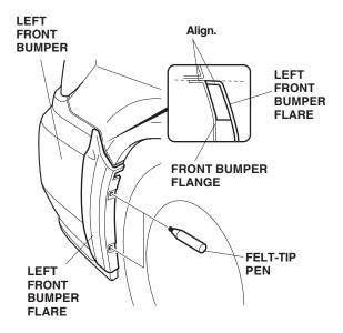
Pierce the left front bumper with a self-tapping screw at the marks. Remove the screw then slide one spring nut over each of the two holes you made in the front bumper.
