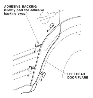
38. Repeat steps 1 through 37 to install the fender flares on the right side of the vehicle.
