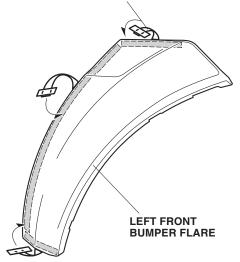
5. Position the left front bumper flare on the front bumper and install the two self-tapping screws (from the kit) through the front bumper. Do not tighten the self-tapping screws yet.
