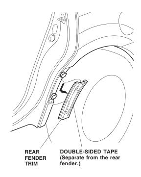
18. Remove and discard the two clips from the rear fender.
