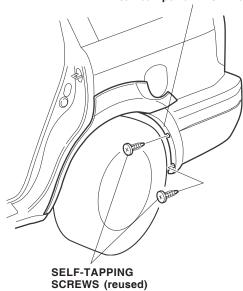
28. Reinstall the molding over the rear fender and fender flange.
