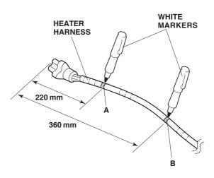
6. Plug the connector end of the heater harness into the engine block heater. Align the A mark you just made on the heater harness with the end of the vehicle connector and secure the heater harness to the vehicle connector with a wire tie.
