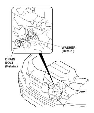
While wearing heavy gloves, install the new aluminum washer and the engine block heater into the bolt hole using a 24 mm socket and a torque wrench. Torque the engine block heater to 60 N⋅m (44 lb-ft).
