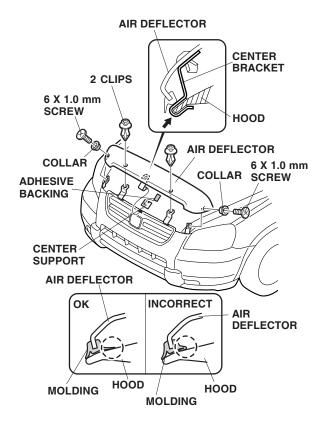
17. Position the air deflector on the hood by sliding the center bracket over the protective tape on the hood, and aligning the holes in the air deflector over the four brackets. Install the two screws, two collars, two clips, and then tighten the screws securely. 18. Open the hood. Reinstall the seal.
