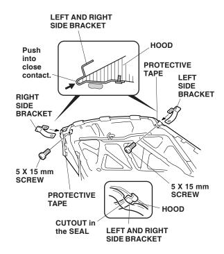
11. Reinstall the two front brackets over the hood around the protective tapes, and install the 5 x 15 mm screws, do not tighten at this time. Push the front brackets against the hood. Insert the front brackets between the seal and hood.
