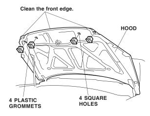
3. Clean the front edge of the hood with one of the alcohol pads included in the kit.
