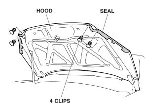
2. Locate the four outer square holes on the inside of the hood. Push a plastic grommet into each of the four outer square holes in the hood.
