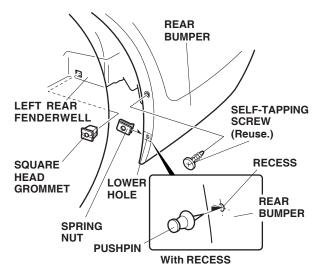
Install one square head grommet into the hole in the left rear fenderwell. Slide one spring nut over the hole you made in step 8 in the rear bumper.  Position the left rear splash guard on the left rear fenderwell and rear bumper, and loosely install one self-tapping screw you removed, and the two selftapping screws supplied with the kit.
